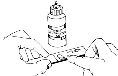
Apply a liberal amount of M-Prep Neutralizer 5A to the gage area. Keeping the surface wet, scrub with cotton-tipped applicators. Do not allow evaporation of the cleaning material on the specimen surface since this would leave a thin, unwanted film between the adhesive and the specimen.
