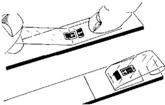
Lift the gage end of the tape assembly as shown here at a shallow angle to the specimen surface (about 45 degrees) until the gage and terminal are free of the specimen surface.
