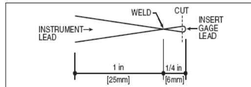
Insert gage lead between the 0.25 inch (6 mm) end of the transition ribbons, and spot weld the two layers of Nichrome at a minimum of three points.
