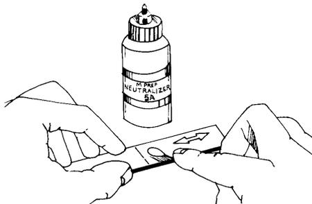
Apply a liberal amount of M-Prep Neutralizer 5A to the gage area. Keeping the surface wet, scrub with cotton-tipped applicators. Do not allow evaporation of the cleaning material on the specimen surface since this would leave a thin, unwanted film between the adhesive
