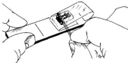
Coat back of gage with the prepared adhesive. A mixing rod can be used to apply a thin layer of adhesive. Be careful not to pick up any unmixed components of the adhesive. To ensure this, it is advisable to wipe the mixing rod clean and then pick up a very small amount of the adhesive from the center area of the adhesive mix. Immediately after coating with the adhesive, proceed
