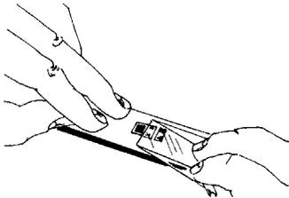
The gage and terminal strip are now solidly bonded in place. To remove the tape, pull it back directly over itself, peeling it slowly and steadily off the surfaces.
