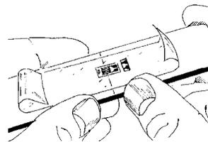
Position the gage/tape assembly so the triangle alignment marks on the gage are over the layout lines on the specimen. Holding the tape at a shallow angle, wipe the assembly onto the specimen surface.
