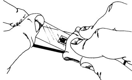
Lift the tuckered-over end of tape and bridge it over the adhesive at approximately a 30-degree angle. With a piece of gauze, slowly make a single wiping stroke over the gage/tape assembly, bringing the gage back down over the alignment marks on the specimen. Use a firm pressure with your fingers when wiping over the gage, since the adhesive is quite viscous. A very thin layer of adhesive is desired for optimum bond performance.
