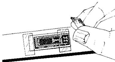
Return the gage/terminal assembly to its original position over the layout marks. Use only enough pressure to allow the assembly to be tacked down. Overlay the gage/ terminal area with a piece of thin Teflon sheet (TFE-1). If necessary, anchor the Teflon in position across one end with a piece of mylar tape.
