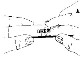
Remove the gage/tape/terminal assembly by peeling tape at a shallow angle (about 30°) and transferring it onto the specimen. Make sure gage alignment marks coincide with specimen layout lines. If misalignment does occur, lift the end of the tape at a shallow angle until assembly is free. Realign and replace. Use of a pair of tweezers often facilitates this handling.
