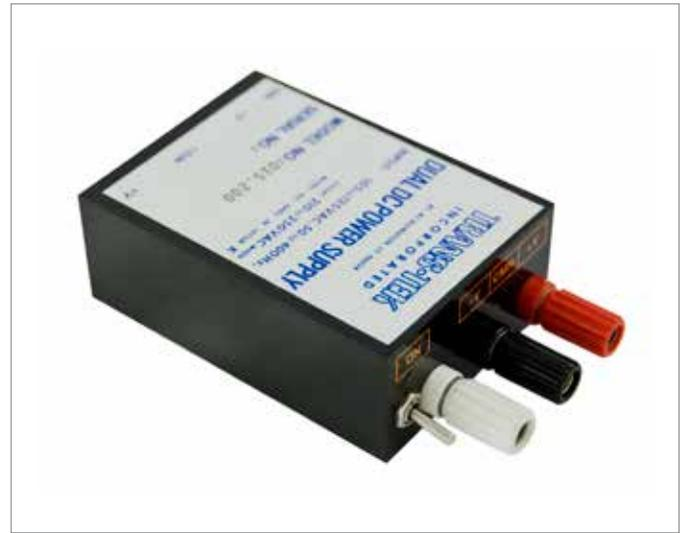
Dual voltage power supplies allow the user to choose the transducer excitation voltage; for example, Model D12.200 can be used to power a transducer with 12 VDC or 24 VDC. To excite the transducer with 12 VDC, connect the transducer +INPUT and -INPUT to the power supply +V and COM terminals, respectively (or to the power supply COM and -V terminals, respectively). To excite the transducer with 24 VDC, connect the transducer +INPUT and -INPUT to the power supply +V and -V terminals, respectively.
