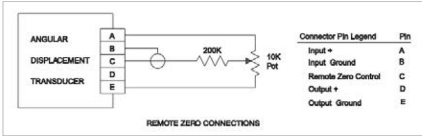
Unless operating in a noise free environment, the lead to pin C must be shielded, as shown. The existing zero adjust potentiometer in the Angular Displacement Transducer must be rotated fully clockwise before the remote zero control can function correctly. This remote function is useful in applications where it is inconvenient to access the adjustment screw on the transducer housing.
