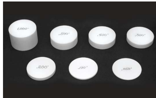
Calibration spacer set 26U-51U (0.050, 0.100, 0.200, 0.300, 0.400, 0.500, 1.000) 850859-001
