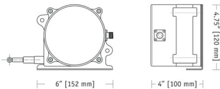
The SR1E is rugged, low-cost, high performance string pot built to withstand wet environments and outdoor applications. Designed for construction equipment and factory use, the SR1E is the perfect low-cost solution for OEM and stocking distributors.
