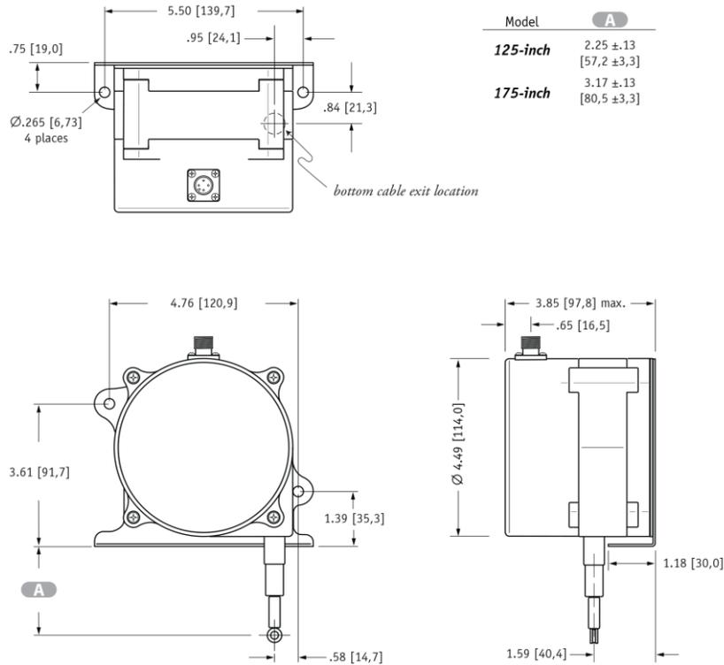
**Fig. 4 - "Rear" Cable Exit Direction**
