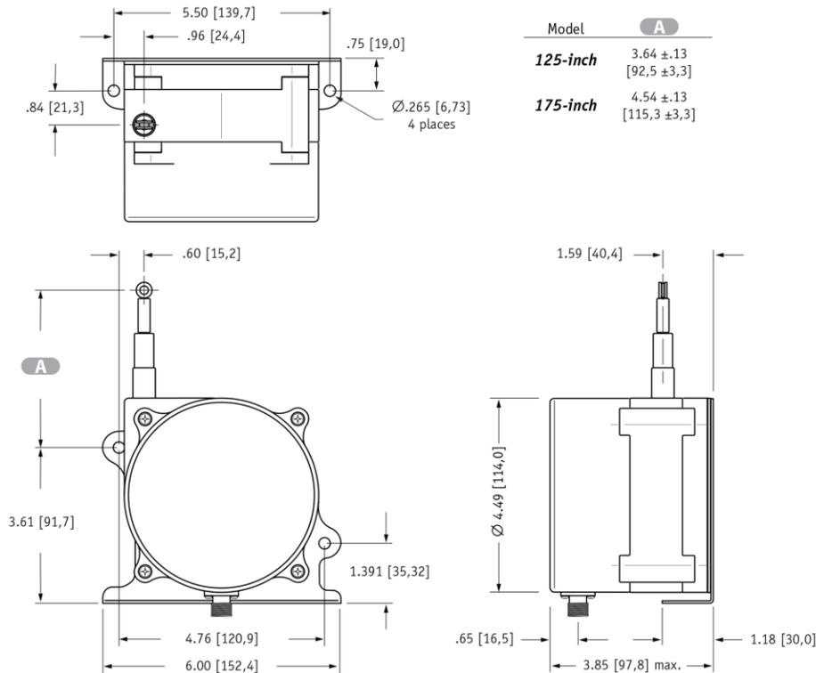
**Fig. 3 - "Down" Cable Exit Direction**
