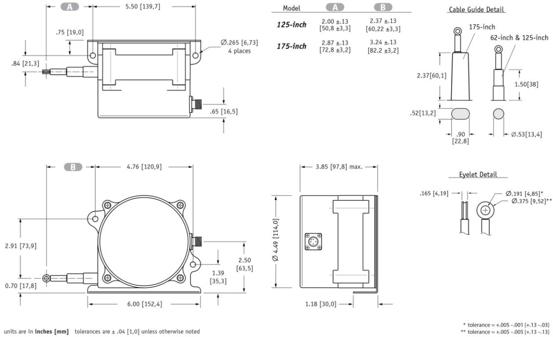
**Fig. 2 - "Up" Cable Exit Direction**
