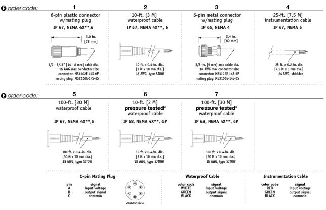
Notes:  $\begin{cases} * -Test pressure: 100 feet [30 meters] H_2O (40 PSID); Test Medium: Air; Duration: 2 hours. * -NEMA 4X applies to stainless steel enclosure only.$
