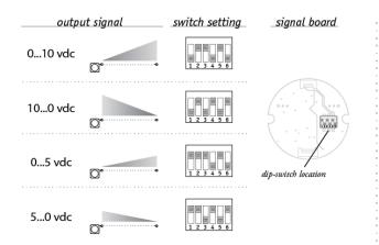
The output signal direction can be reversed at any time by simply changing the dip-switch settings found on the internal signal board. After the settings have been changed, adjustment of the Zero and Span trimpots will be required to precisely match signal values to the beginning and end points of the stroke.
