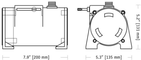
The PT9301 is a combination position and velocity transducer for demanding long-range applications requiring a linear position measurements in ranges up to 1700". A precision plastic-hybrid potentiometer provides accurate position feedback while a self-generating DC tachometer provides a velocity signal that is proportional to the speed of the traveling stainless-steel measuring cable.
