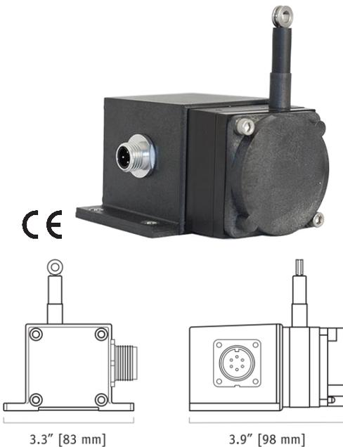
The PT1DC can operate from an unregulated 14.5 to 40 VDC power supply while providing an output signal that is proportional to the linear movement of its measuring cable. The PT1DC has a maximum measurement range up to 50" and has 4 output signal options to choose from: 0...10, 0...5, -10...+10 and -5...+5 Vdc.
