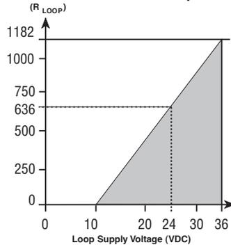
$$V_{min} = 10V + (.022A \times R_L)$$
