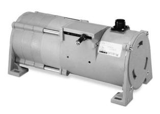
The PT9DN communicates via DeviceNET protocol with programmable controllers in factories and harsh environments requiring linear position measurements in ranges up to 1700".
